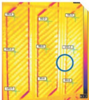
Figure 2 Hot area in a single stage setter.
