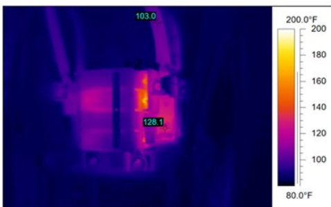
Figure 3. Thermal image of main circuit breaker after installation of cooling fan.
