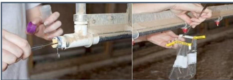
Figure 2. Taking swab and drip samples to monitor the residual and microbial efficacy of water treatment
